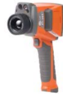
Figure 1.4 A thermal camera used to find cold spots in a leaky house. Source: Passivhaus Institut " http://en.wikipedia.org/wiki/File:SONEL_KT-384.jpg ." Used under BY-SA 3.0 //creativecommons.org/licenses/by-sa/3.0/deed.en.
